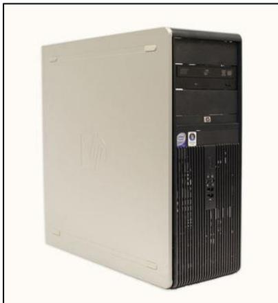
The **computer case** is the metal and plastic box that **contains the main components** of the computer. It houses the motherboard, central processing unit (CPU), power supply, and more.
